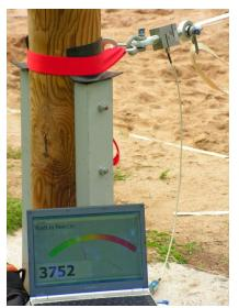
exercise lesson. Of special interest here was the installation of the force sensor in so-called Jumplines, at which surprisingly high forces of approx. 9 kN were reached very fast.
